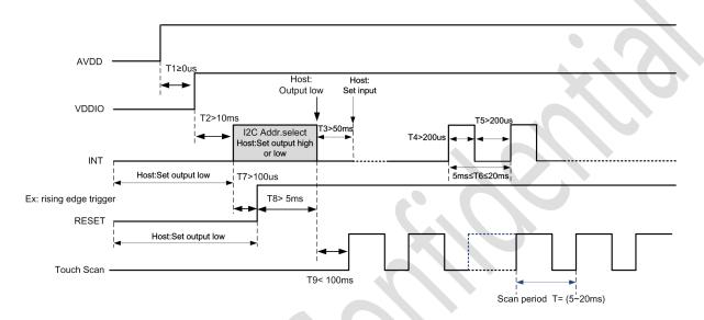
Whether host outputs high or low after INT T2 depends on which I<sup>2</sup>C slave address the host employs to communicate with GT911. If the address is 0x28/0x29, host outputs high; if the address is 0xBA/0xBB, host outputs low.
