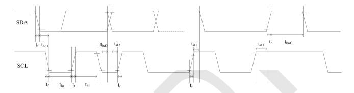
Test condition 1: 1.8V host interface voltage, 400Kbps transmission rate,  $2K\Omega$  pull-up resistor
