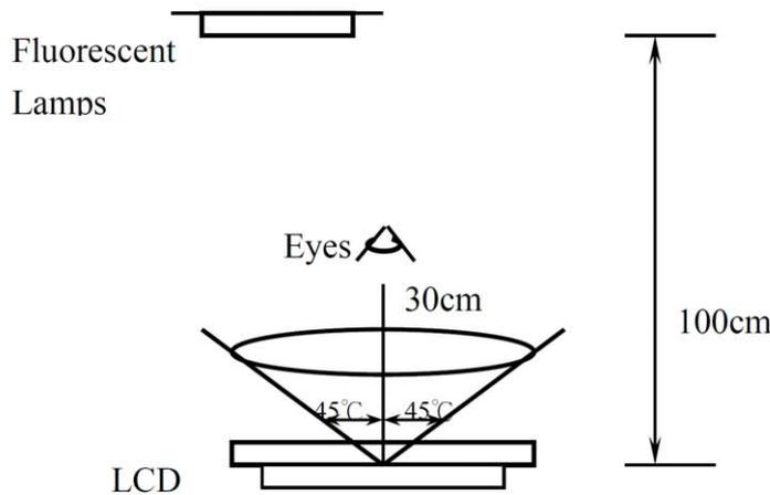
6.4.1.2 When test the model of transmissive product must add the reflective plate.
