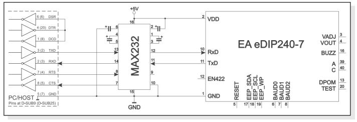
Application example to direct pc interfacing
