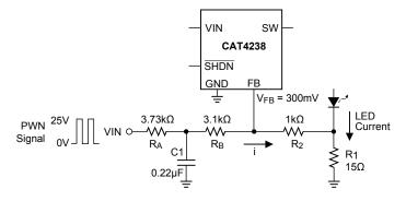
Figure 2. Circuit for Filtered PWM Signal
