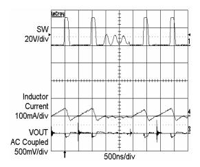
Switching Waveform VIN = 5.0V,  $I_{LED} = 1.5mA$
