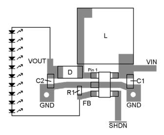
Figure 5. Recommended PCB Layout
