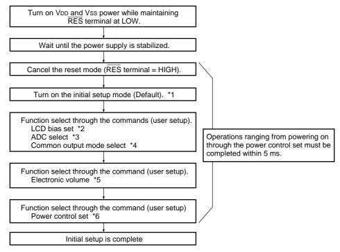
\* This duration of 5 ms depends on the panel characteristics as well as capacity of the capacitor concerned.
