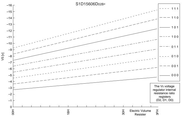
Figure 14: S1D15606D02B\* (3) For models with External Input
