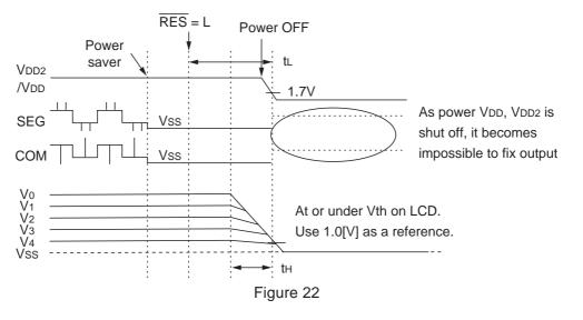
S1D15B01D00B\* has the discharge faculty that is shorted VOUT to VDD2, when RES pin=LOW. As tH0=70(µs/V), Δ tH=0.079(µs/V/nF) by measurement, tH is calculated as follows, when V0=7V and CL=100pF. tH=tH0×V0+Δ tH×CL×V0=70×7+0.079×100×7=545µs
