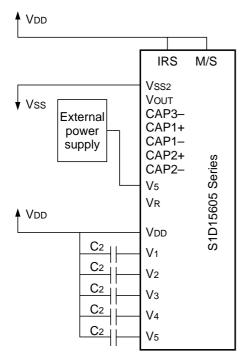
(5) When the built-in power circuit is used to drive a liquid crystal panel heavily loaded with AC or DC, it is recommended to connect an external resistor to stabilize potentials of V1, V2, V3 and V4 which are output from the built-in voltage follower.
