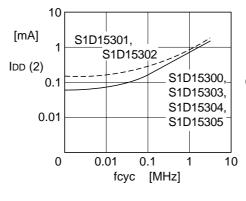
This indicates current consumption when data is always written on the checker pattern at fcyc. When no access is made, only IDD (1) occurs.
