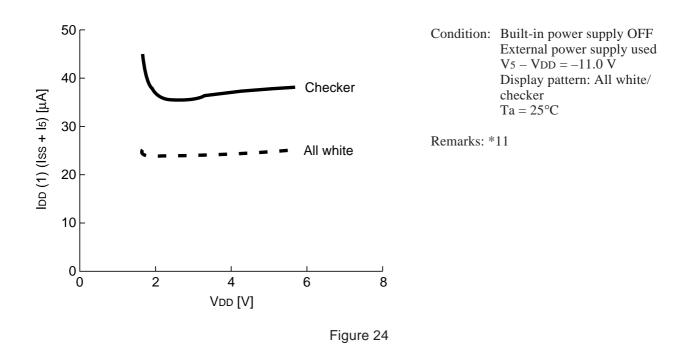
[Reference data 2] • Dynamic current consumption (2) Built-in power supply used and LCD being displayed
