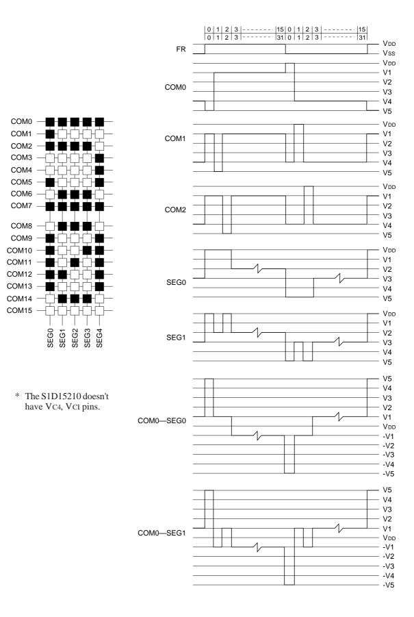
Figure 4 LCD drive waveforms example
