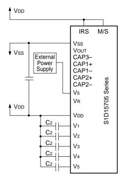
(4) Only the external power supply used Depending on all external power supplies
