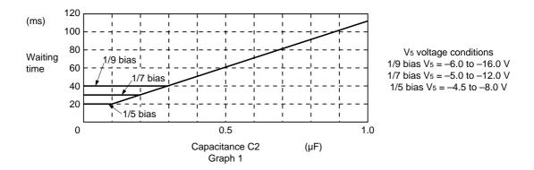
\*5: Within the waiting time in built-in power supply ON status, any command other than built-in power supply control commands such as Power Save, and display ON/OFF command, display normal rotation/reverse command, display all ON command, output status select command and DUTY+1 clear command can accept another command without any problem. RAM read and write operations can be freely performed.
