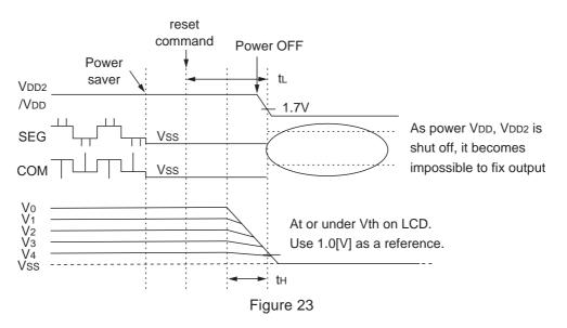
Vout is not shorted to VDD2 by reset command, so th is longer than the case of  $\overline{\text{RES}}$  pin=LOW. As th0=175( $\mu$ s/V),  $\Delta$  th=0.23( $\mu$ s/V/nF) by measurement, th is calculated as follows, when V0=7V and CL=100pF. th=th0×V0+ $\Delta$  th×CL×V0=175×7+0.23×100×7=1386 $\mu$ s
