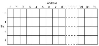
Each 8-bit display data byte loaded from the command/ data register is stored in two consecutive addresses as shown in the following figure. The upper four bits are stored at the location specified by the address counter, and the lower four bits, at the next location. The address counter is automatically incremented by two.
