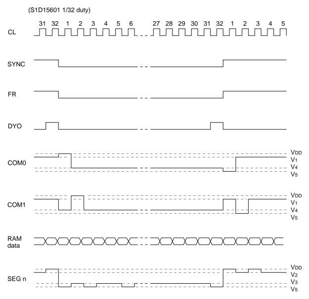
Figure 7. Frame driver timing
