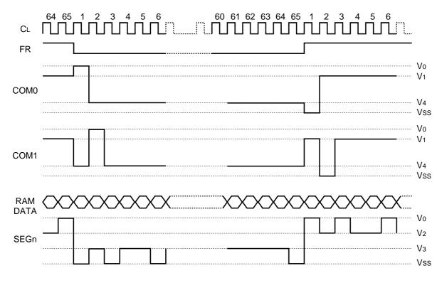
2-frame AC drive waveforms
