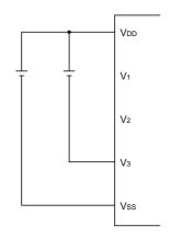
Figure 2. LCD drive supply not connected to Vss
