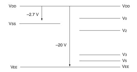
4. If the logic power is being floated or if the Vss voltage exceeds -2.5 Vdc during LCD power-on, the LSI chips may be damaged permanently. Take care not to damage the chips especially in the system power on/off sequence.
