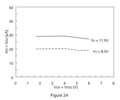
Conditions : Internal power supply OFF. External supply in use. V0=8.0V, Display pattern : Checker, Ta=25°C
