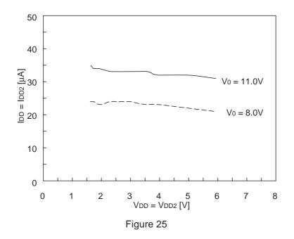
Dynamic current consumption (2): During display, when the internal power supply circuit is ON.
