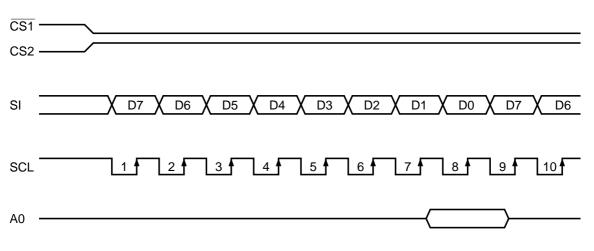
Figure 1. Serial interface timing
