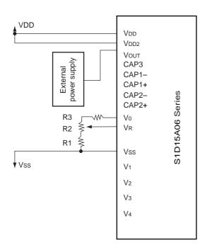
(2) When built-in V<sub>0</sub> voltage adjusting resistors are used Voltage Follower Circuit [S1D15A06D01B\*]
