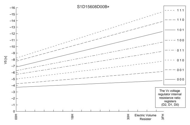
Figure 18: S1D15608D00B\* (1) For Models Where the Thermal Gradient = -0.05%/°C
