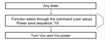
The time spent for the operations ranging from power save through powering off (VDD – VSS = 2.4V) (tL) must be longer than the time required for V5 to V1 go under the LCD panel threshold voltage (normally 1V). \* tH is determined by time constant of the external resisters Ra and Rb (for adjusting voltages V5 to V1) and the smoothing capacitor C2. \* It is recommended to cut tL shorter by connecting a resistor between VDD and V5.
