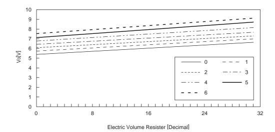
Figure 9 The V<sub>0</sub> voltage as a function of the V<sub>0</sub> voltage regulator internal resister internal resistor and the electronic volume register [Ta=25°C]
