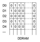
As is shown in Figure 3, the D7 to D0 display data from the MPU corresponds to the LCD common direction.
