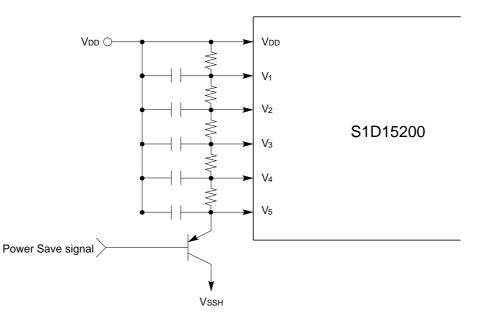
If the LCD drive power is generated by resistance division, the resistance and capacitance are determined by the LCD panel size. After the panel size has been determined, reduce the resistance to the level where the display quality is not affected and reduce the power consumption using the divider resistor.
