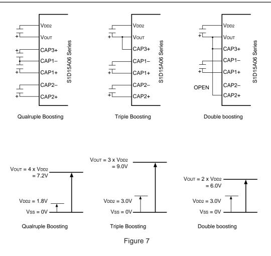
\*VDD2 voltage must be set so that VOUT voltage does not exceed the absolute maximun rated value.
