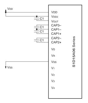
(2) When built-in V<sub>0</sub> voltage adjusting resistors are not used (When VDD2 = VDD boosted 4 times)
