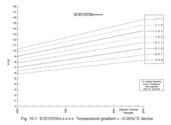
$V_5$  voltage based on the values of  $V_5$  voltage adjusting built-in resistance ratio register and electronic control register
