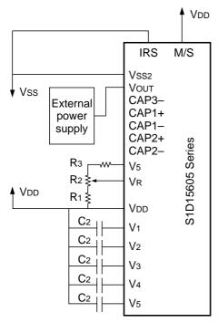
(2) When the V5 voltage regulator internal resistor is used.
