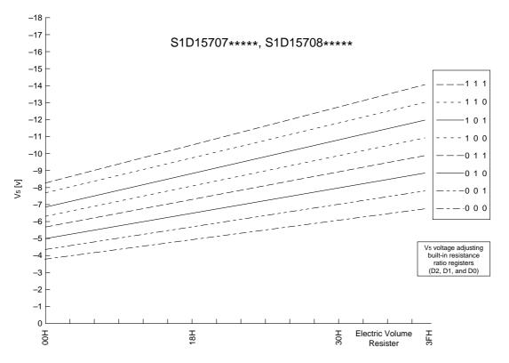
Fig. 10-2 S1D15707\*\*\*\*\*, S1D15708\*\*\*\*\* Temperature gradient = -0.05%/°C device
