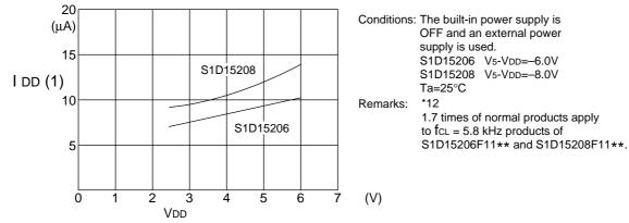
• Dynamic current consumption (2) when the LCD built-in power supply lamp is ON
