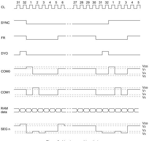
Figure 8. Line inverse driver timing
