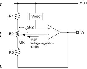
To use the Electronic Volume Control Function, issue the Set Power Control command to simultaneously operate both the voltage regulator circuit and voltage follower circuit.
