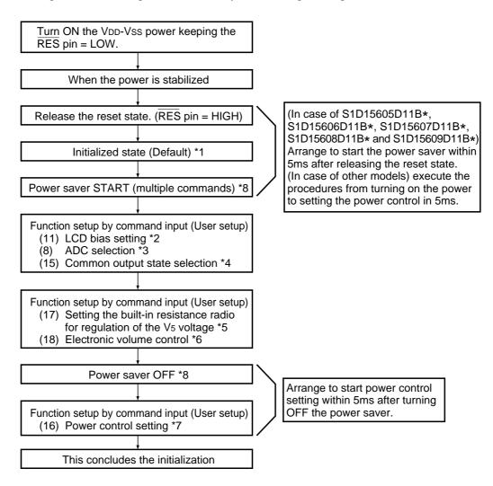
\* The target time of 5ms will result to vary depending on the panel characteristics and the capacitance of the smoothing capacitor. Therefore, we suggest you to conduct an operation check using the actual equipment.
