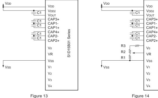
(2) When used only the voltage regulator circuit and V/F circuit [S1D15B01D01B\*]
