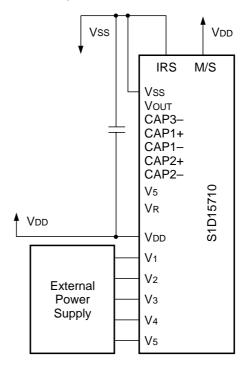
Common reference setting example At V5=-8 to -12 V variable
