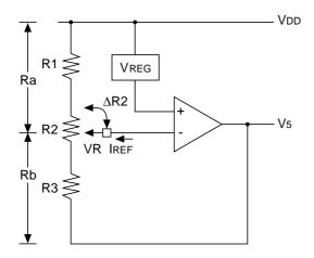
$V_{REG}$  is the constant voltage source of the IC, and in case of Type 1, it is constant and  $V_{REG} = -2.55$  V (if  $V_{DD}$  is 0 V). In case of Type 2,  $V_{REG} = V_{SS}$  ( $V_{DD}$  basis). To adjust the  $V_5$  output voltage, insert a variable resistor between  $V_R$ ,  $V_{DD}$  and  $V_5$  as shown. A combination of R1 and R3 constant resistors and R2 variable resistor is recommended for fine-adjustment of  $V_5$  voltage.
