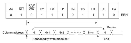
Cancels read-modify-write mode and restores the contents of the column address register to their value prior to the receipt of the read-modify-write command.
