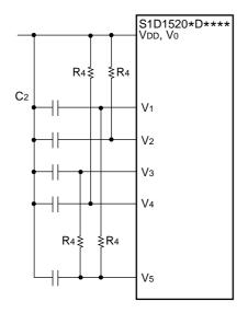
Note: Use jumper and shielded wires as the input impedance of VR terminal is high.
