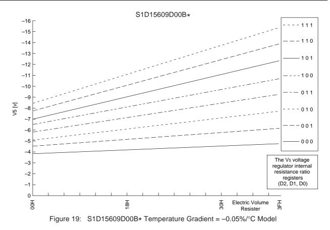
Setup example: When selecting  $Ta = 25^{\circ}C$  and V5 = 7 V for an S1D15607 model on which Temperature gradient =  $-0.05\%/^{\circ}C$ .
