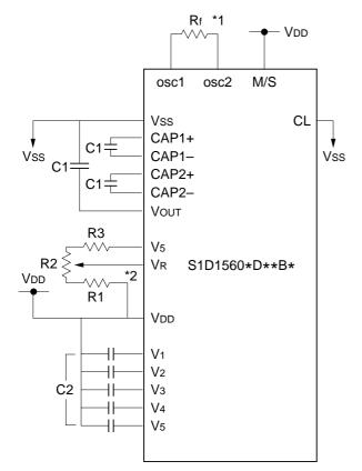
When the built-in power circuit is used
