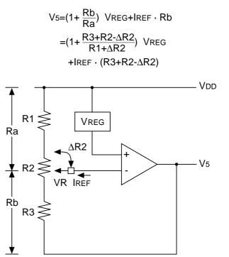
$V_{REG}$  is the constant voltage source of the IC, and it is constant and  $V_{REG}$ =-2.5 ± 0.15 V (if  $V_{DD}$  is 0 V). To adjust the V<sub>5</sub> output voltage, insert a variable resistor between V<sub>R</sub>, V<sub>DD</sub> and V<sub>5</sub> as shown. A combination of R1 and R3 constant resistors and R2 variable resistor is recommended for fine-adjustment of V<sub>5</sub> voltage.
