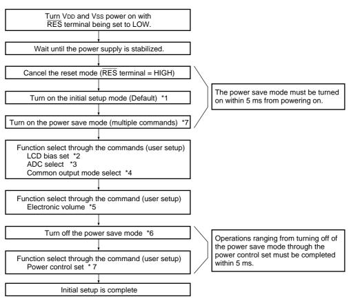
\* This duration of 5 ms depends on the panel characteristics as well as capacity of the capacitor concerned. Check them on the actual system.
