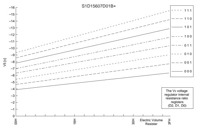
Figure 16: S1D15607D01B\* (2) For Models Where the Thermal Gradient = -0.2%/°C
