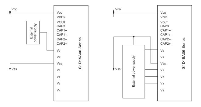
\* Since VR pin has a higher impedance, wiring distance must be minimized or shielded wire must be used.
