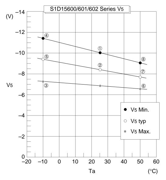
Example of V<sub>5</sub> Voltage When Using S1D15600/601/602 Series Electronic Volume
