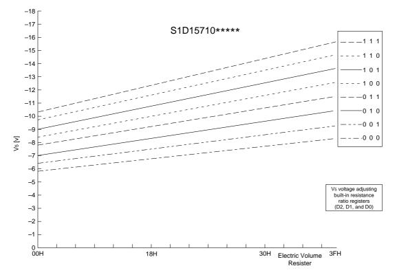
Figure 10 S1D15710\*\*\*\*\* Temperature gradient = -0.05%/°C
