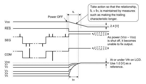
If command control is disabled when power is OFF, take action so that the relationship,  $t_L > t_H$ , is maintained by measures such as making the trailing characteristic of power (VDD – VSS) longer.
