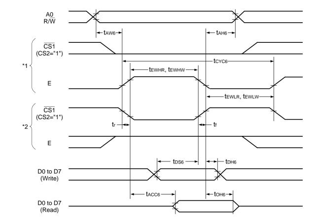
System bus read/write characteristics 2 (68 series MPU)
