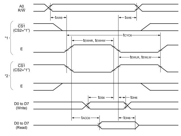
System bus read/write characteristics 2 (68 series MPU)
