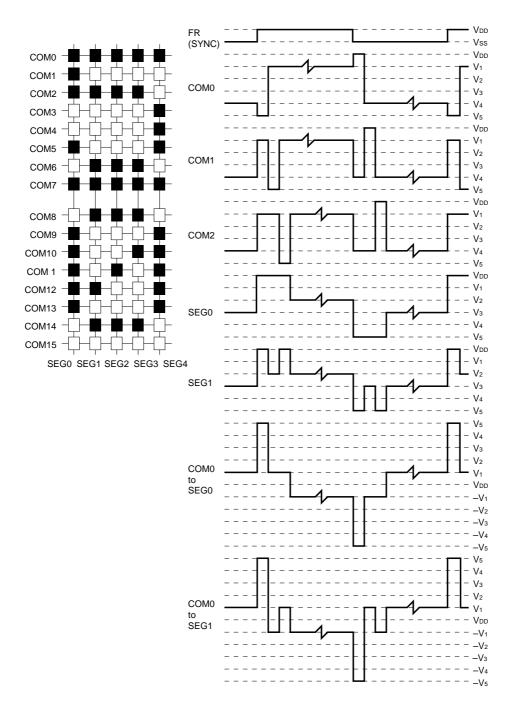
Figure 9. Example of segment and common timing
