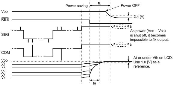
Set up tL so that the relationship, tL > tH, is maintained. A state of tL < tH may cause faulty display.
