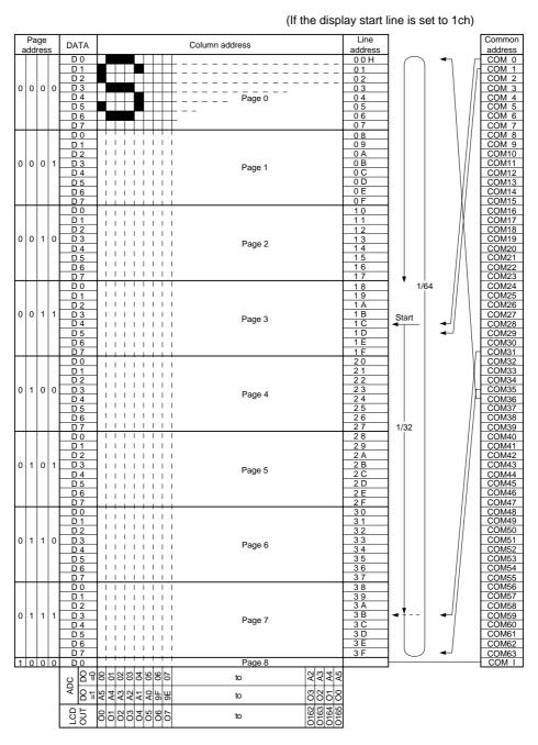
Figure 4. Display data RAM addressing
