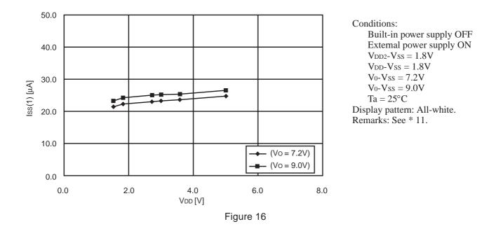
◊ Dynamic operating current (1) - When LCD display is turned on with external power supply being connected (Checker pattern display)
