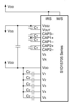
(2) When not using the V5 voltage adjusting built-in resistor (Example of Vss2=Vss, quadruple boosting)
