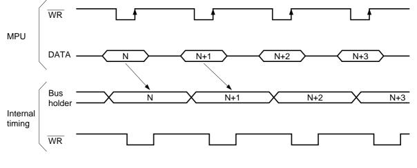
Figure 2. Write timing
