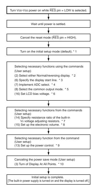
on the display screen during its powering on process. In order to avoid such troubles, it is recommended to implement the following flow.
