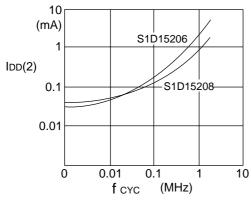
It shows the current consumption when a checker pattern is always written in fSYNC timing. When not accessed, only the current consumption of IDD (2) occurs.
