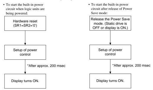
\* When the Set Power Control command is issued, the V  $_{DD}$  level signal is output at both COM and SEG terminals for approximately 200 msec. Any other command can be entered during this period.
