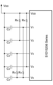
the resistance of ITO wiring is being inserted in series with the switching transistor, thus dominating the boosting ability. Consequently, the boosting ability will be hindered as a result
