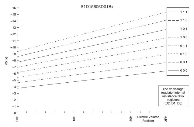
Figure 13: S1D15606D01B\* (2) For Models Where the Thermal Gradient = -0.2%/°C
