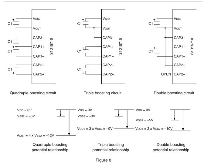
• Set the VSS2" voltage range so that the voltage of the VOUT pin cannot exceed the absolute maximum ratings.
