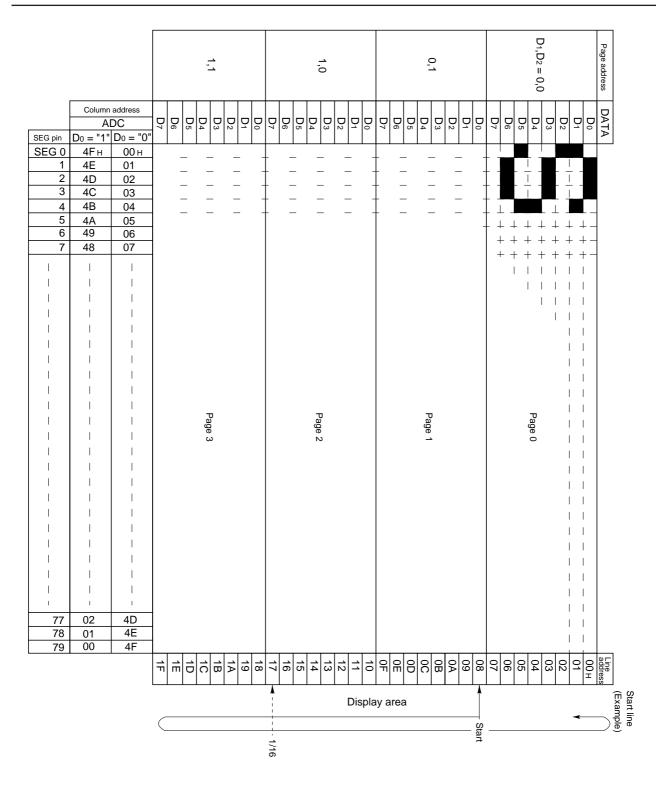
Figure 2 Display Data RAM Addressing
