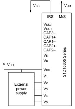
Examples of shared reference settings When V<sub>5</sub> can vary between -8 and 12 V
