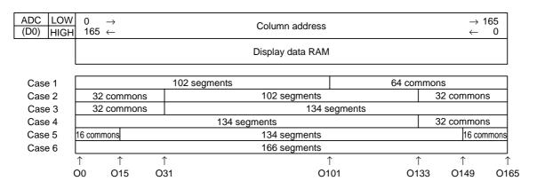
Figure 6. Output configuration selection
