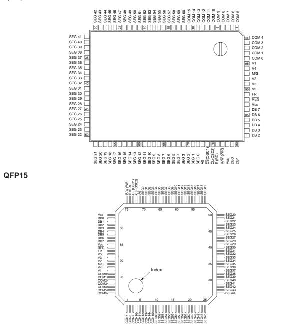
Note: This is an example of S1D15200F pin assignment. The modified pin names are given below.
