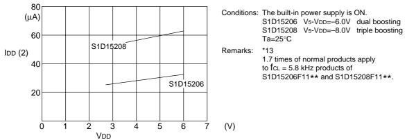
Current consumption I DD during access (2) during MPU access cycle
