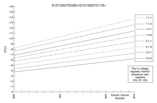
Figure 15: S1D15607D00B\*/S1D15607D11B\* (1) For Models Where the Thermal Gradient = -0.05%/°C
