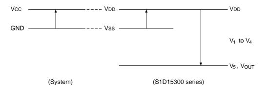
Notes: 1. V1 to V5, V<sub>OUT</sub>, voltages are based on V<sub>DD</sub>=0 V.
