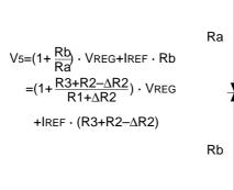
where,  $V_{REG}$  is the constant voltage source of the IC, and it is constant ( $V_{REG} = -3.1$  V). ( $V_{REG} = Type1$ )  $V_{REG} = V_{SS}(V_{DD} \text{ basis})$  ( $V_{REG} = Type2$ )
