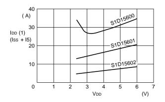
Conditions: The built-in power supply is off but the external one is used. S1D15600  $V_5 - V_{DD} = -12.5 V$ S1D15601  $V_5 - V_{DD} = -8.0 V$ S1D15602  $V_5 - V_{DD} = -6.0 V$ External clock: S1D15600 fcL = 4 kHz S1D15601 fcL = 2 kHz S1D15602 fcL = 1 kHz Remarks: \*14
