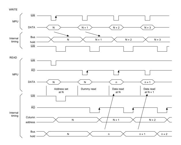
Figure 1 Bus Buffer Delay
