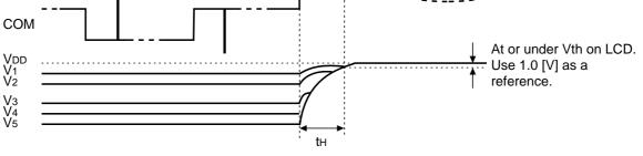
If command control is disabled when power is OFF, take action so that the relationship,  $t_L > t_H$ , is maintained by measures such as making the trailing characteristic of power (VDD – VSS) longer.
