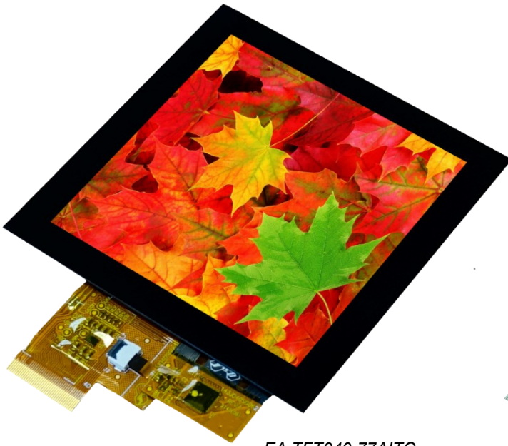
EA TFT040-77AITC Dimension 94x94x3.8mm Image similar
