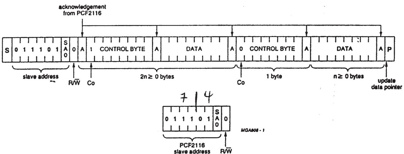
Master transmits to slave receiver; WRITE mode.
